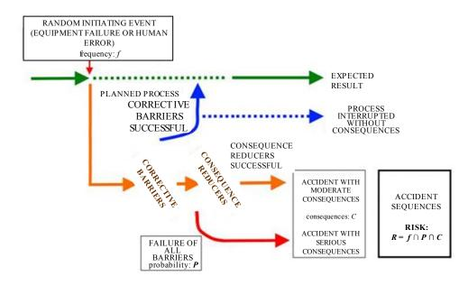
FIG. 1. Typical accidental exposure sequence.
